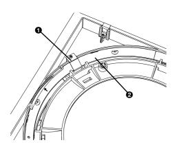
If the angle adjustment ring is out of true in the cover, the ring must be repositioned.
