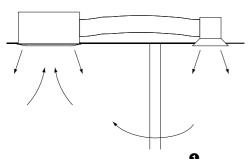
The CC has a prepunched hole in the casing. A Ø160 mm air duct can be mounted to this hole, so that discharge air can be led to an additional air grille.
