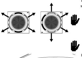
The discharge pattern can be adjusted to the room using the supplied blind plates.
