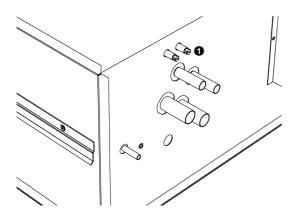
The vent valve • is above the CH connections. The CC HI/C2 has two vent valves.
