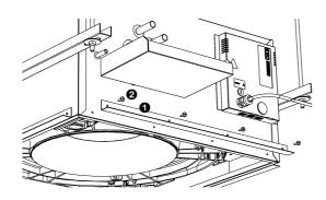
If the unit is integrated into a suspended ceiling, the ceiling tiles should not rest on the cover. For correct installation, you may want to use the optional edge sections.
