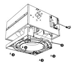
6. Remove the drip tray 2 using screws 3.
