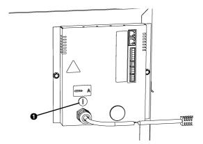
The unit's electronics module has one fuse. The fuse rating is specified on a sticker near the fuse.
