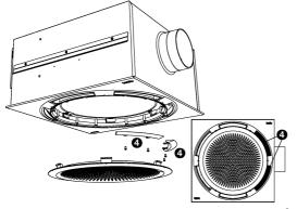
5. Mount the two supplied blind plates 4 into the discharge grille, on the side of the air connection (see section 2.14)
